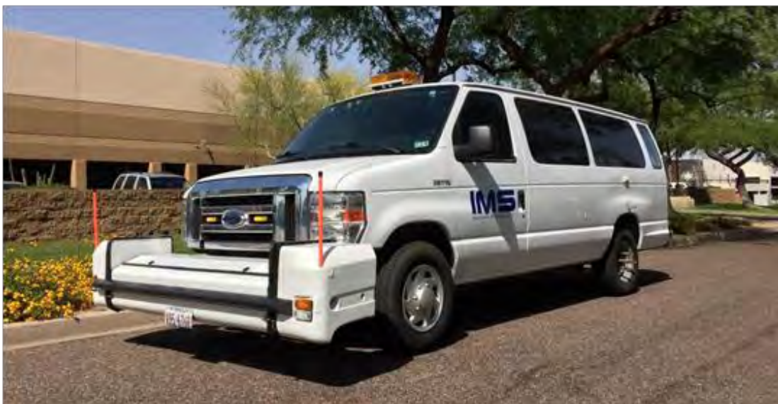
Figure 4 – Laser Road Surface Tester (RST)
